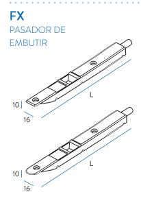
L: 150 mm 200 mm 250 mm 300 mm  $400 \, \text{mm}$ 500 mm
